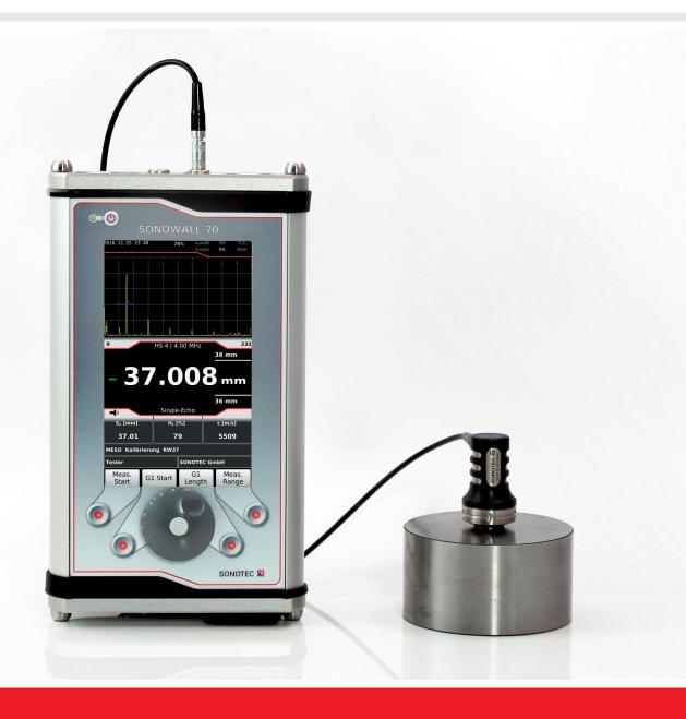
**ULTRASONIC A-SCAN/B-SCAN THICKNESS GAUGE**
